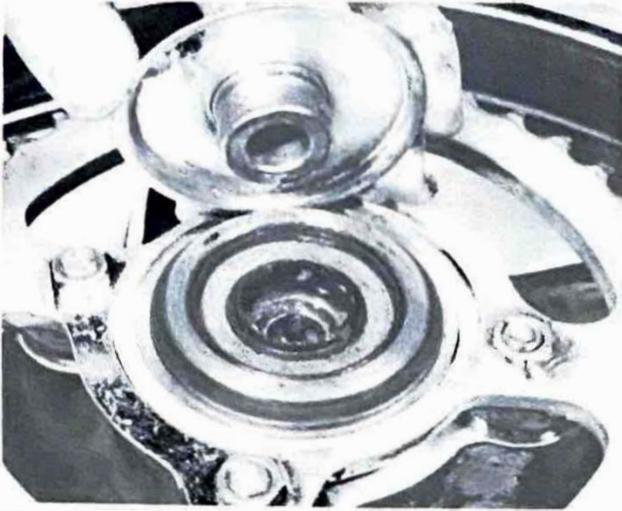
12.1a Remove flanged spacer ...
