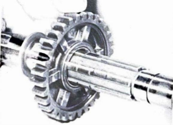
14.7b Fit the 2nd gear pinion with engagement webs as shown
