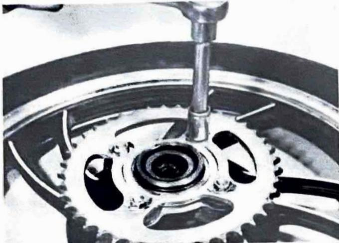
14.2c ... the four sprocket retaining nuts
