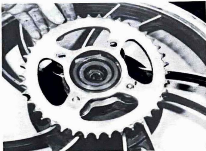
14.2d Sprocket can now be removed ...
