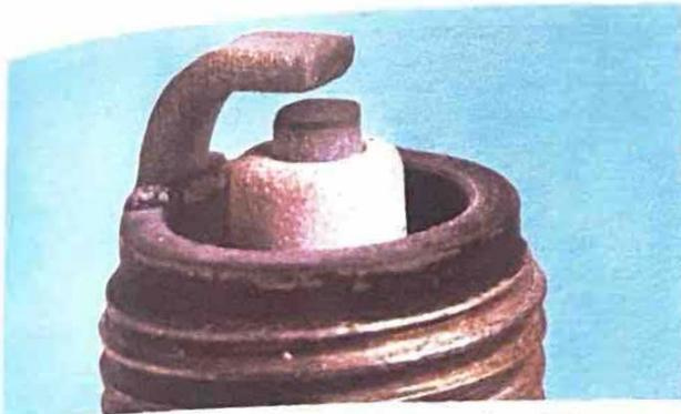
Spark plug conditions: A brown, tan or grey firing end is indicative of correct engine running conditions and the selection of the appropriate heat rating plug
