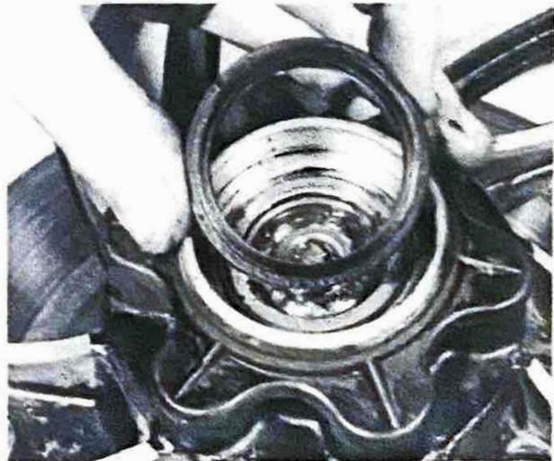
11.1b ... and prise out grease seal
