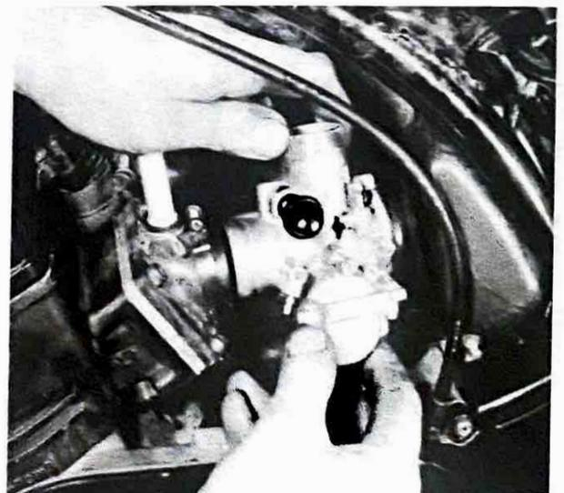
4.8b Slacken clips and disengage carburettors from stubs
