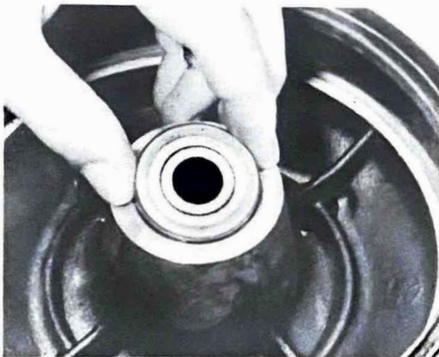
12.1c Fit bearing with sealed face outwards ...
