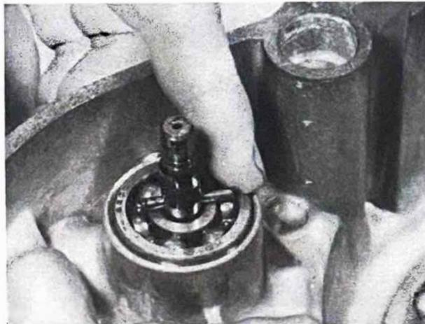
7.2c ... then displace drive pin from shaft end
