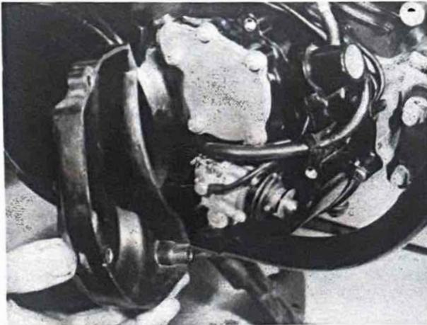
7.2a Water pump is mounted above oil pump
