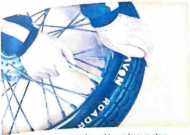
**Tyre removal:** Deflate inner tube and insert lever in close proximity to tyre valve
