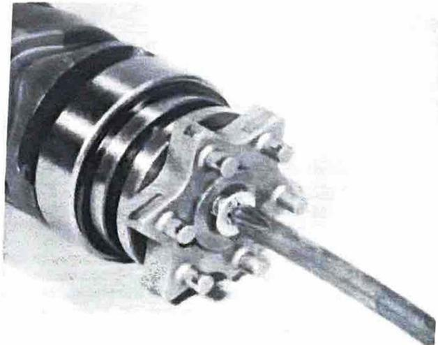
20.8a Camplate is retained by a single cross-head screw
