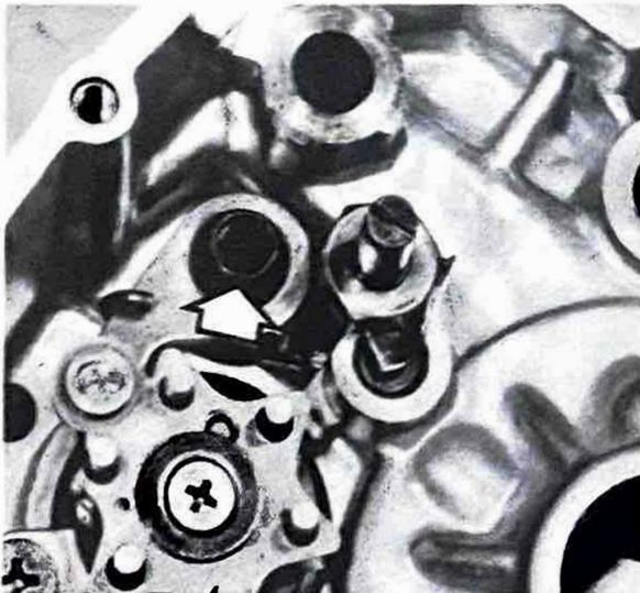
12.3a Remove pivot bolt and lift stopper arm away
