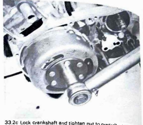
33.2c Lock crankshaft and tighten nut to prescribed torque
