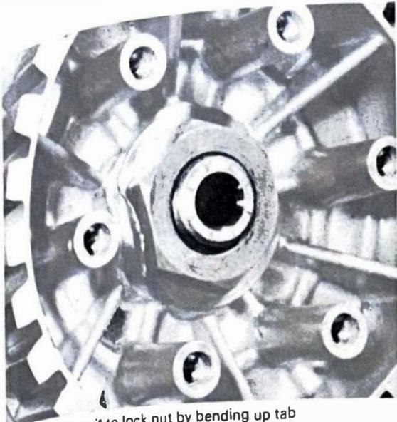
32.3g Do not omit to lock nut by bending up tab
