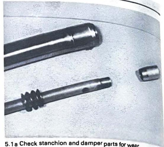
5.1 a Check stanchion and damper parts for wear
