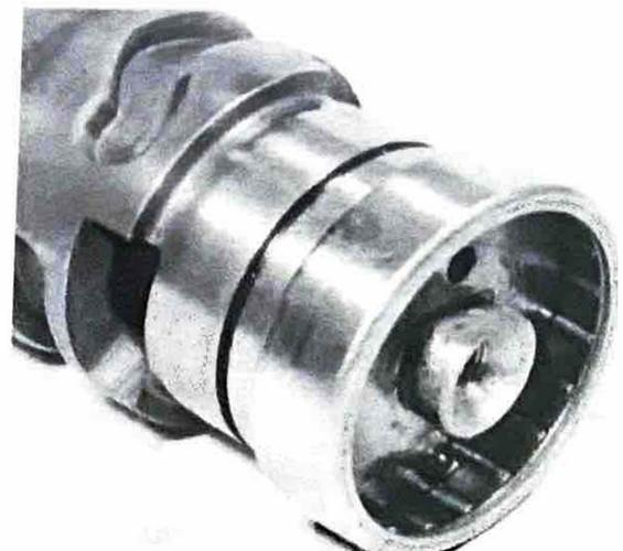
20.8c ... and slide the caged needle-roller bearing off
