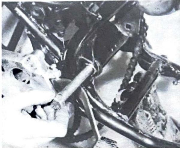
10.3c Remove nut and withdraw the pivot shaft ...
