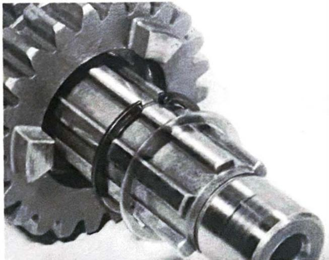
14.5c Position circlip in next groove, then fit washer
