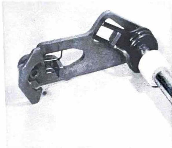
30.2a Check that the selector claw and springs are positioned as shown ...
