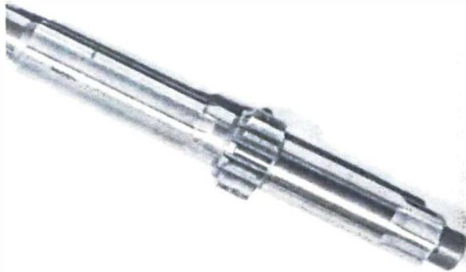
14.4a 1st gear pinion is integral with input shaft
