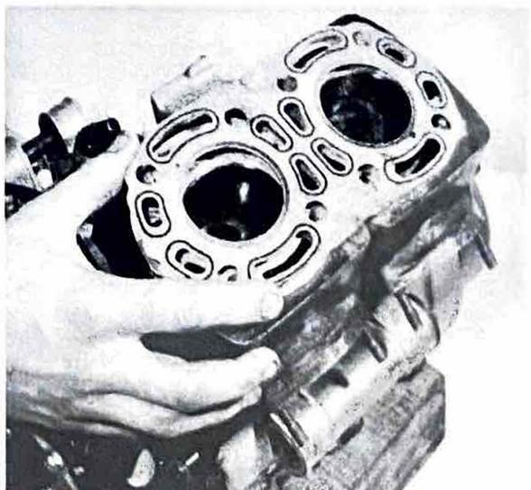
34.5a Place a new cylinder head gasket in position ...
