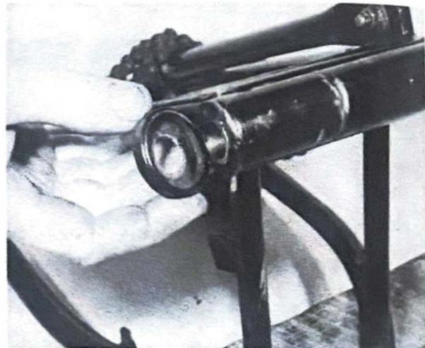
10.4 Remove end covers, noting any shims fitted
