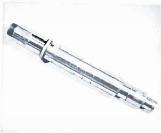
14.7a Output shaft has plain shoulder at sprocket end
