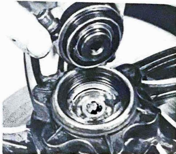
11.1a Remove speedometer drive gearbox ...
