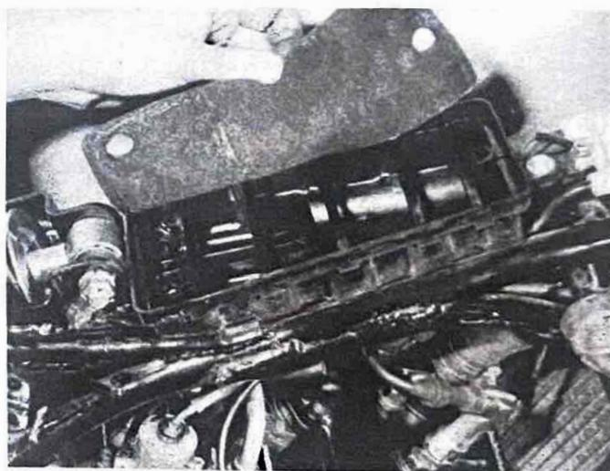
12.3b Filter element can be removed for cleaning
