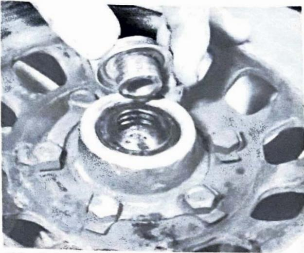
11.1e Moving to RH side, remove headed spacer ...
