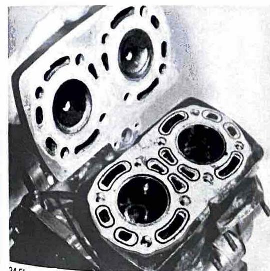
34.5b ... then lower cylinder head into place
