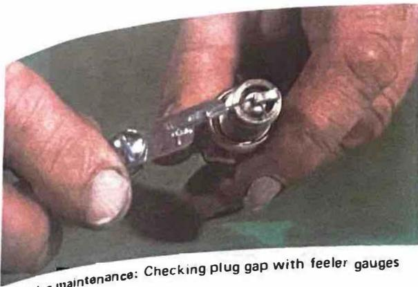
Spark plug maintenance: Checking plug gap with feeler gauges
