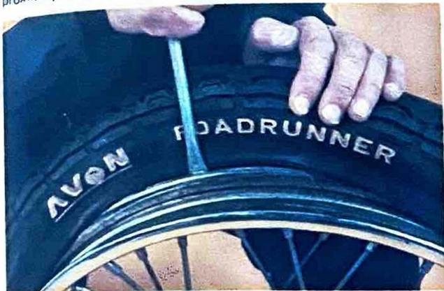
When first bead is clear, remove tyre as shown
