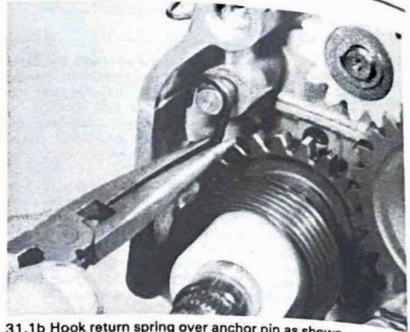
31.1b Hook return spring over anchor pin as shown
