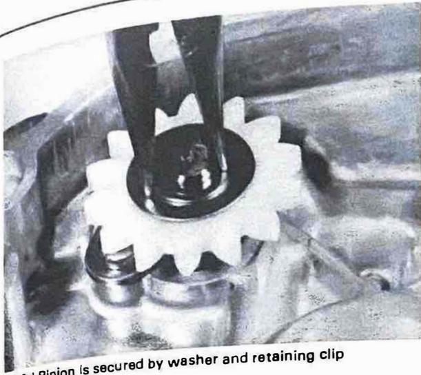
25.2d Pinion is secured by washer and retaining clip
